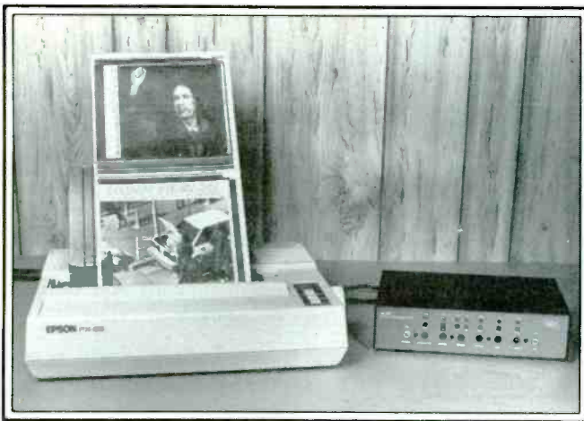
M-800 FAX converter driving Epson FX-85 dot matrix printer. Unit is printing out press wire photo on shortwave bands.
