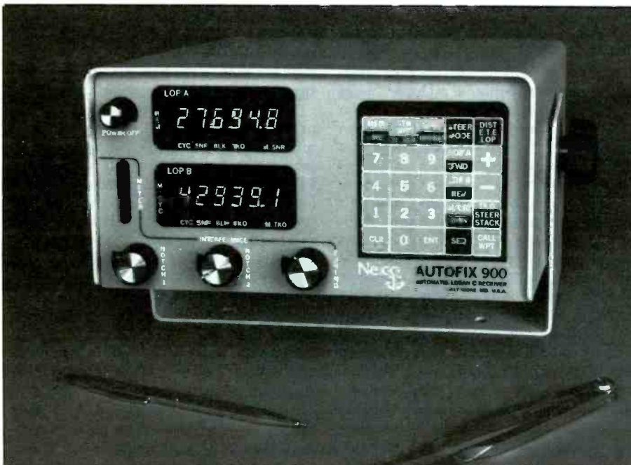
For accurate, instant position determination, use a Loran receiver. Note the very small size of this Autofix 900.
