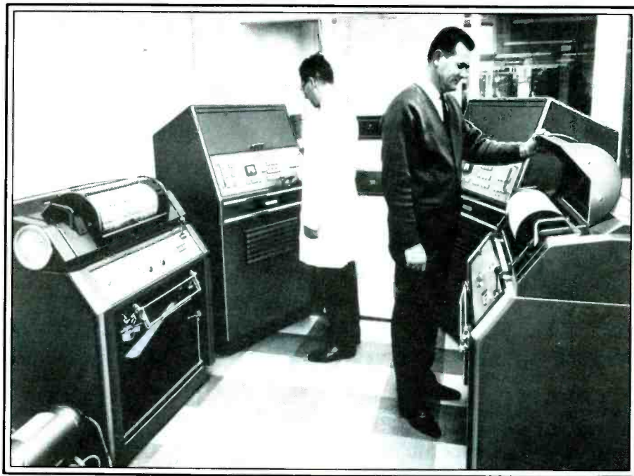
Two large drum Muirhead Industries facsimile machines in newsroom use.
